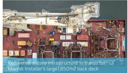
Recovered subsea infrastructure in transit on Maersk Installer's large 1,850m<sup>2</sup> back deck
